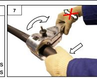
Keep the cable end downwards in order to prevent particles from entering during preparation.
